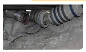
Defective lower support roller of a belt conveyor
